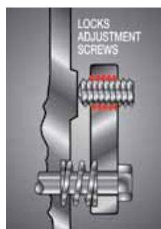
**Locks Adjustment Screws.** This simple design allows permanent, positive adjustment of screws in any position. Secure against vibration or impact.
